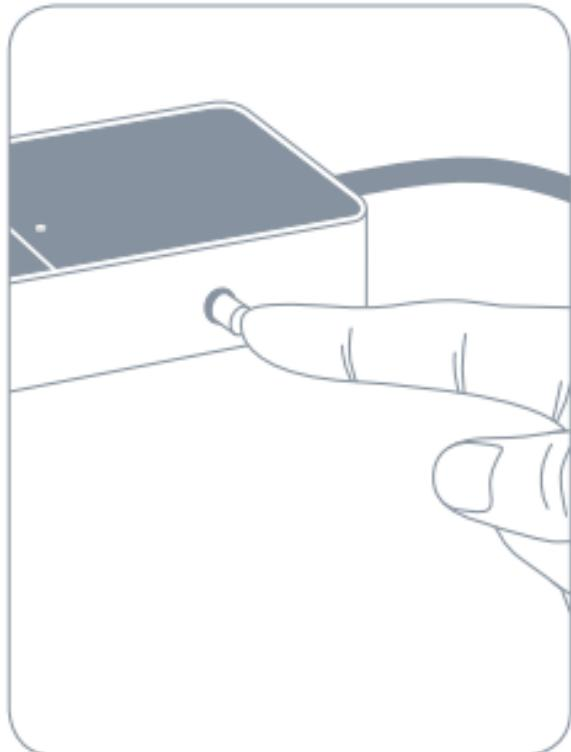
If an electrical surge is detected, the fuse on the side of Eve Energy Strip will eject and the protection indicator LED will turn off. To resume operation, unplug Eve Energy Strip and reinsert the fuse.
